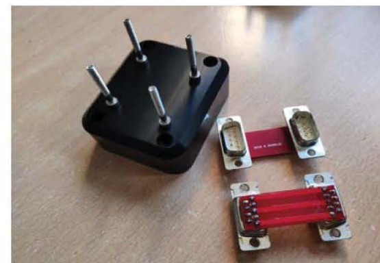
6 pieces of DELRIN HV COVERS with 24 pieces of M3 x 25mm bolts and 6 pieces of 9 pin HV BRIDGES[red PCB]
